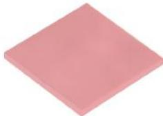
TP600 is a high thermal conductivity material with high conformability at low pressures. It is self-adhesive on both sides. When assembled with electronic components, it exhibits lower thermal resistance and better electrical insulation characteristics under low compression force. It can work stably at -40°C~150°C and meet the flame retardant rating requirements of UL94 V0.
