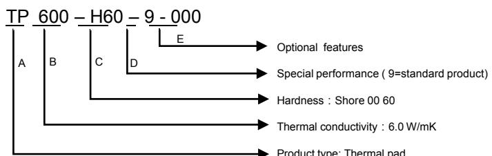
Standard size: 200x400mm. May be die cut into various sizes or shapes according to customer's specifications. The thickness selected should be 15 to 20% thicker than highest tolerance gap to ensure material fills all voids and wets out mating surfaces.
